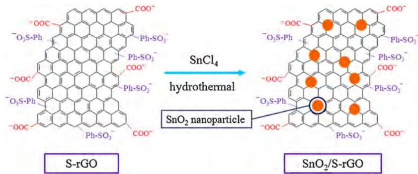
Fig. 1. A scheme to illustrate the modification of S-rGO with SnO<sub>2</sub> nanoparticles by hydrothermal synthesis method.
