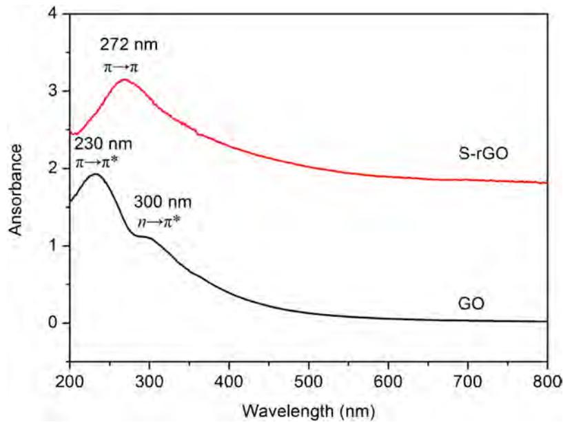
Fig. 2. UV-vis spectra of GO and S-rGO.
