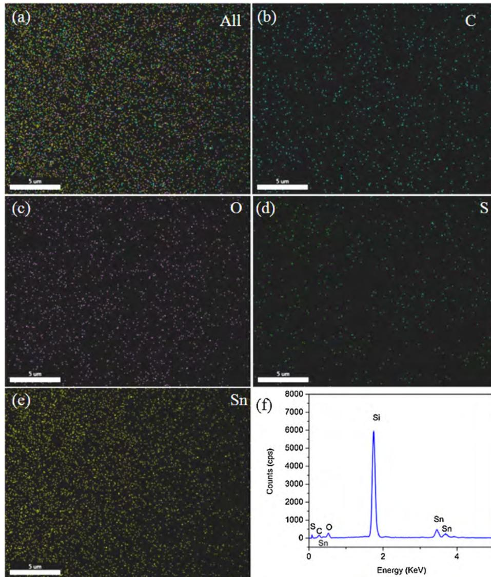
Fig. 5. The EDS mapping for (a) all, (b) C element, (c) O element, (d) S element, (e) Sn element, and (f) corresponding EDS spectrum.
