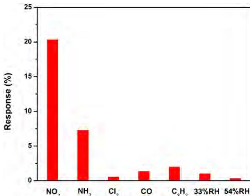
Fig. 11. Comparison of responses of SnO<sub>2</sub>/S-rGO hybrids to various gases at room temperature.
