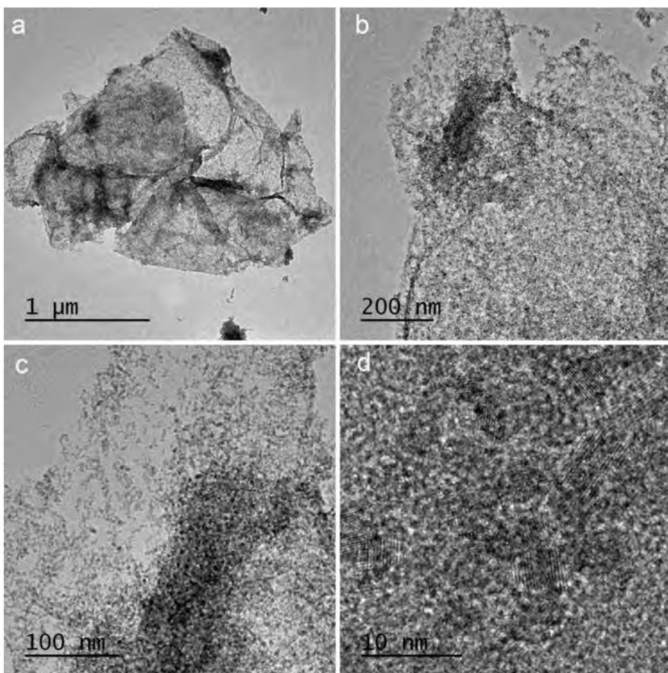
Fig. 6. The TEM images of SnO<sub>2</sub>/S-rGO hybrids.
