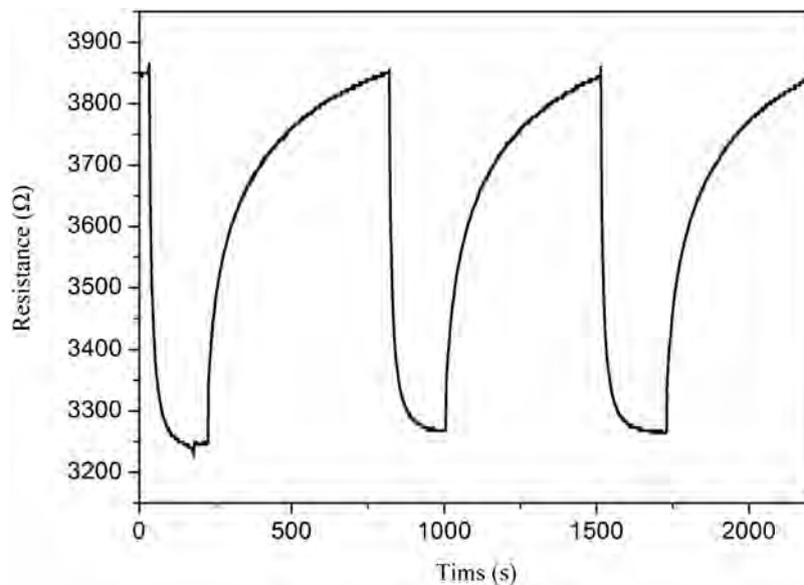
**Fig. 10.** The reproducibility of temporal response of  $\text{SnO}_2/\text{S-rGO}$  hybrids exposed to 5 ppm  $\text{NO}_2$  at room temperature.
