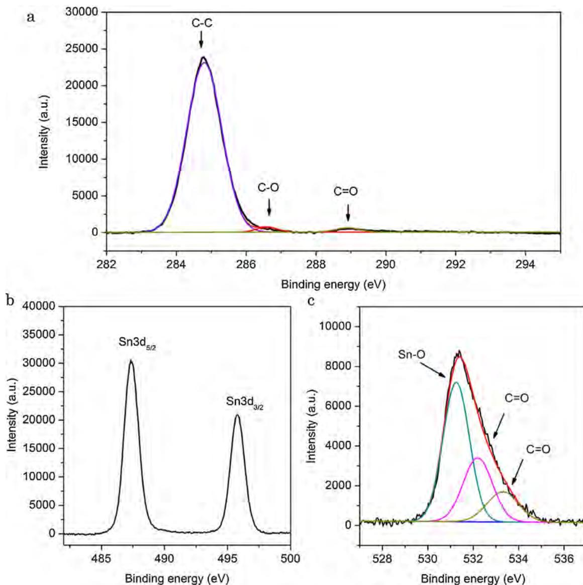
Fig. 3. (a) C1s spectrum, (b) Sn3d spectrum and (c) O1s spectrum of SnO<sub>2</sub>/S-rGO hybrids.
