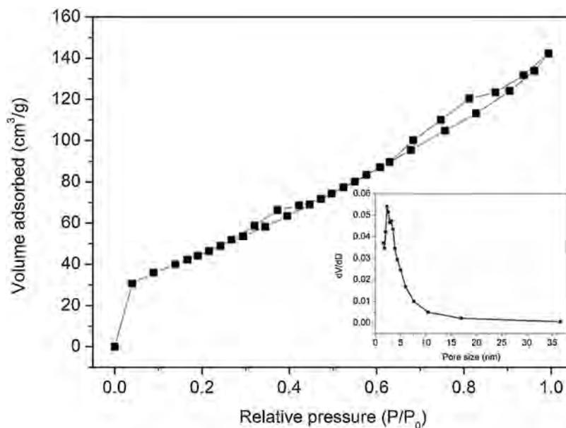
Fig. 7. N<sub>2</sub> sorption isotherms of SnO<sub>2</sub>/S-rGO hybrids. Inset shows the corresponding pore size distribution curve.
