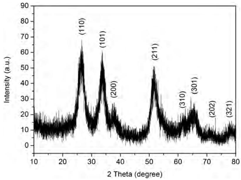
Fig. 4. XRD pattern of SnO<sub>2</sub>/S-rGO hybrids.
