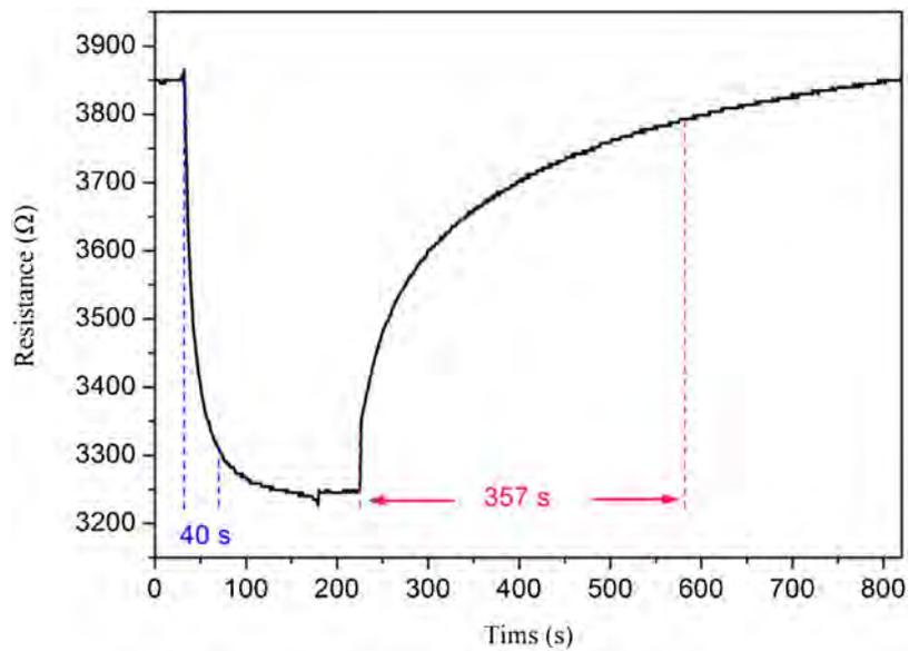
**Fig. 9.** The response and recovery curve of the sensor based on  $\text{SnO}_2/\text{S-rGO}$  hybrids toward 5 ppm  $\text{NO}_2$  at room temperature.
