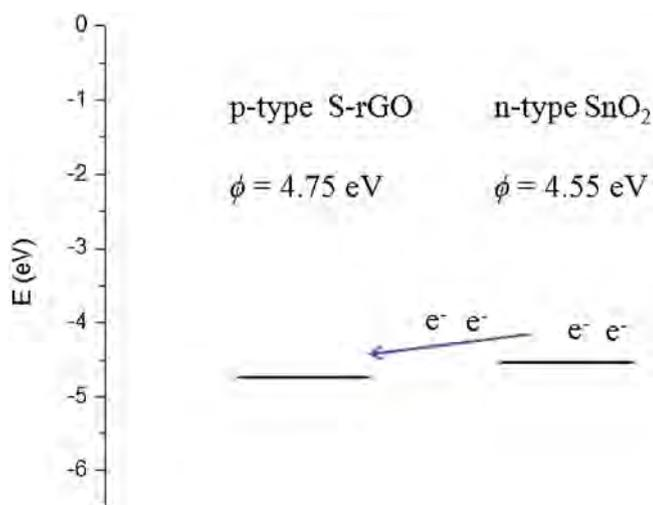
Fig. 12. The scheme to illustrate the electrons transfer progress between S-rGO and SnO<sub>2</sub> during the NO<sub>2</sub> sensing.
