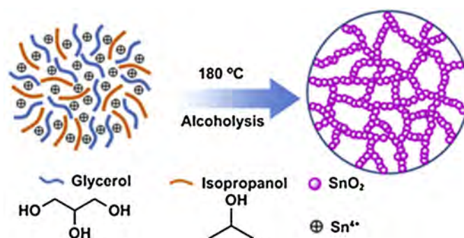
Scheme 2. Preparation of the as-synthesized porous SnO 2 via solvothermal treatment.
