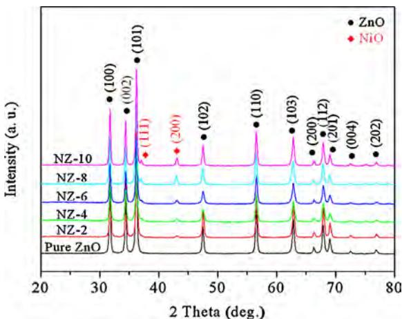
**Fig. 2.** XRD patterns of the pure ZnO and NiO/ZnO nanofibers.
