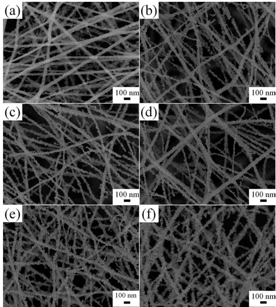
**Fig. 3.** SEM images of the pure ZnO and NiO/ZnO nanofibers: (a) pure ZnO, (b) NZ-2, (c) NZ-4, (d) NZ-6, (e) NZ-8, (f) NZ-10.
