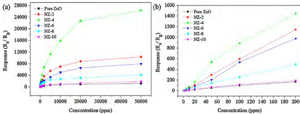
**Fig. 6.** Response of the pure ZnO and NiO/ZnO nanofibers versus TMA concentrations: (a) 0.5–50000 ppm; (b) 0.5–200 ppm.
