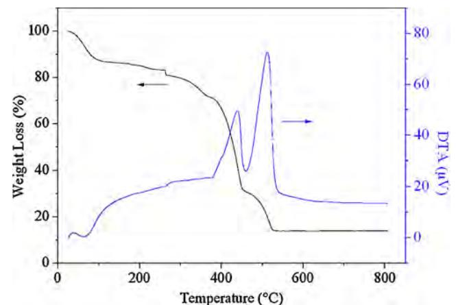
**Fig. 1.** DTA-TGA curves of the Zn(CH<sub>3</sub>COO)<sub>2</sub>/PVP/Ni(CH<sub>3</sub>COO)<sub>2</sub> composite nanofibers.
