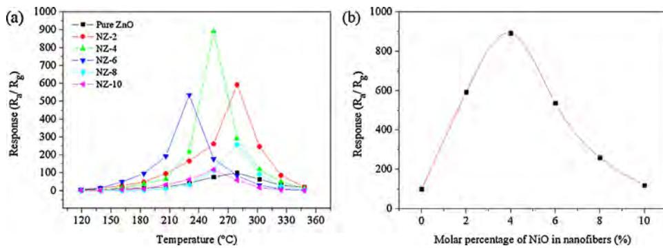
**Fig. 5.** (a) Response of the pure ZnO and NiO/ZnO nanofibers to 100 ppm TMA measured at different operating temperature and (b) response to 100 ppm versus NiO content of nanofibers.
