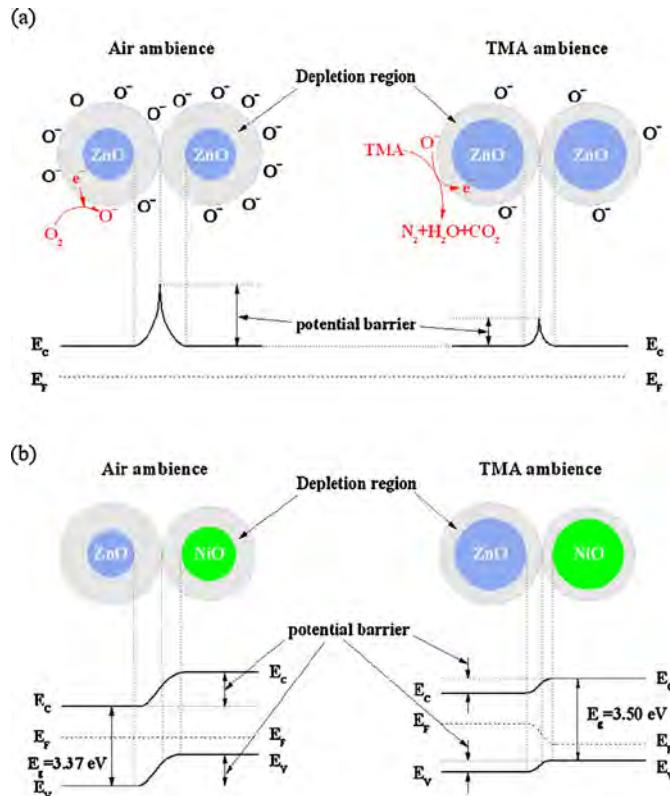
**Fig. 10.** Schematic diagrams of the TMA sensitive mechanism of pure ZnO and NiO/ZnO nanofibers.
