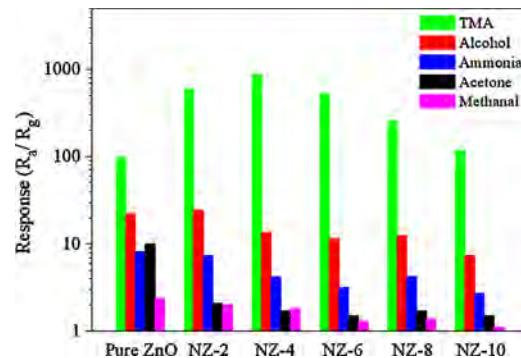
**Fig. 8.** Selectivity and stability of the pure ZnO and NiO/ZnO nanofibers exposed to 100 ppm target gases at their optimal operating temperature.
