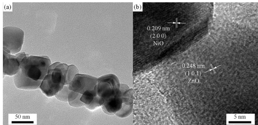
**Fig. 4.** (a) TEM and (b) HRTEM images of p-type NiO/n-type ZnO heterojunction in NZ-4 nanofibers.
