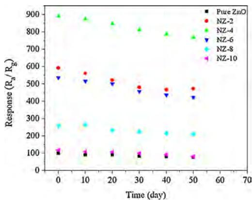
**Fig. 9.** Stability measurement of NiO/ZnO nanofibers to 100 ppm TMA within 50 days.
