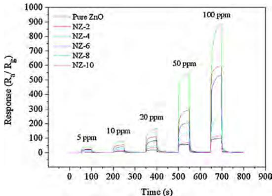
**Fig. 7.** Real-time response curves of the pure ZnO and NiO/ZnO nanofibers to TMA in the range of 5–100 ppm at their optimal operating temperature.
