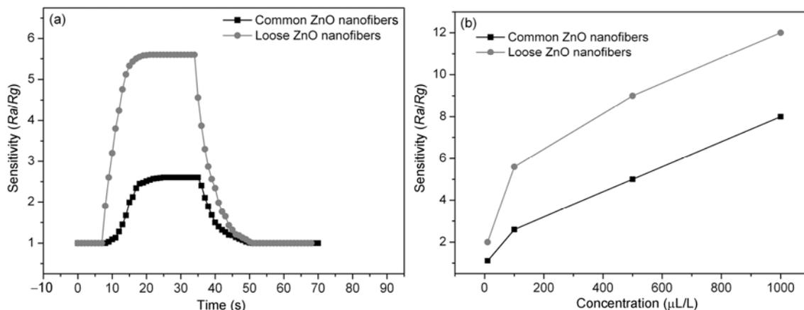
**Figure 7** (a) Response-recovery curves of the sensors fabricated from common and loose ZnO nanofibers to 100 μL/L acetone at 260°C; (b) sensitivities of the sensors fabricated from common and loose ZnO nanofibers to different concentrations of acetone at 260°C.
