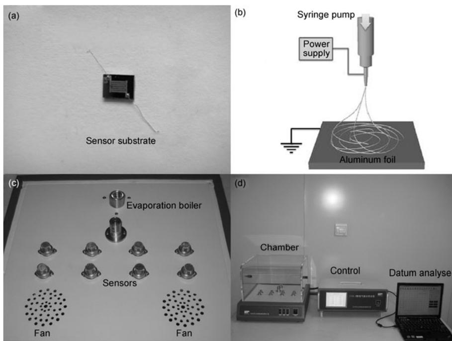
**Figure 2** (a) A photograph of a sensor substrate and a coin; (b) fabricating process of the loose ZnO nanofibers; (c) a photograph of eight micro-sensors in an analysis system; (d) a photograph of the gas sensing analysis system.
