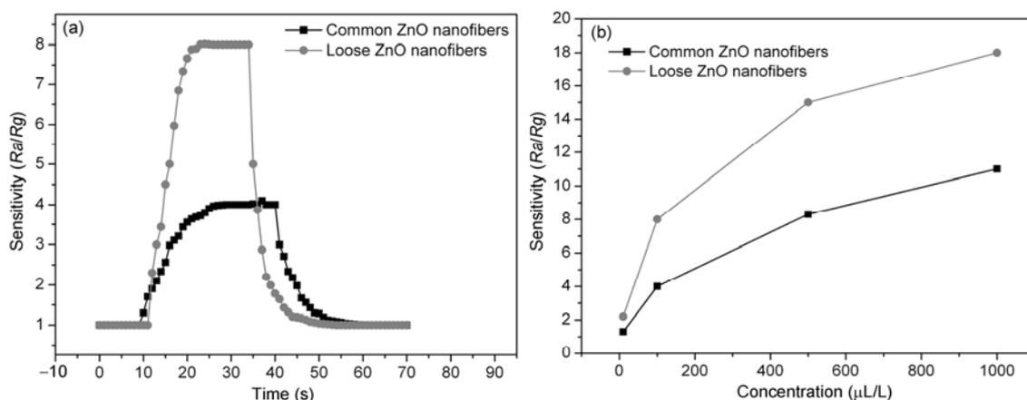
**Figure 6** (a) Response-recovery curves of the sensors fabricated from common and loose ZnO nanofibers to 100  $\mu L/L$  ethanol at 260°C; (b) sensitivities of the sensors fabricated from common and loose ZnO nanofibers to different concentrations of ethanol at 260°C.
