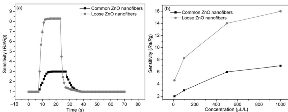
**Figure 8** (a) Response-recovery curves of the sensors fabricated from common and loose ZnO nanofibers to 100 μL/L H<sub>2</sub> at 300°C; (b) sensitivities of the sensors fabricated from common and loose ZnO nanofibers to different concentrations of H<sub>2</sub> at 300°C.
